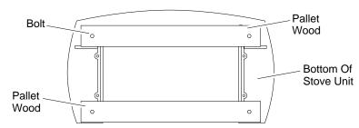
Figure 7 - Removing Pallet Wood From The Bottom of The Stove
